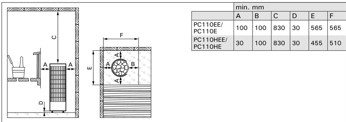
Figure 4. Safety distances (all dimensions in millimeters)
