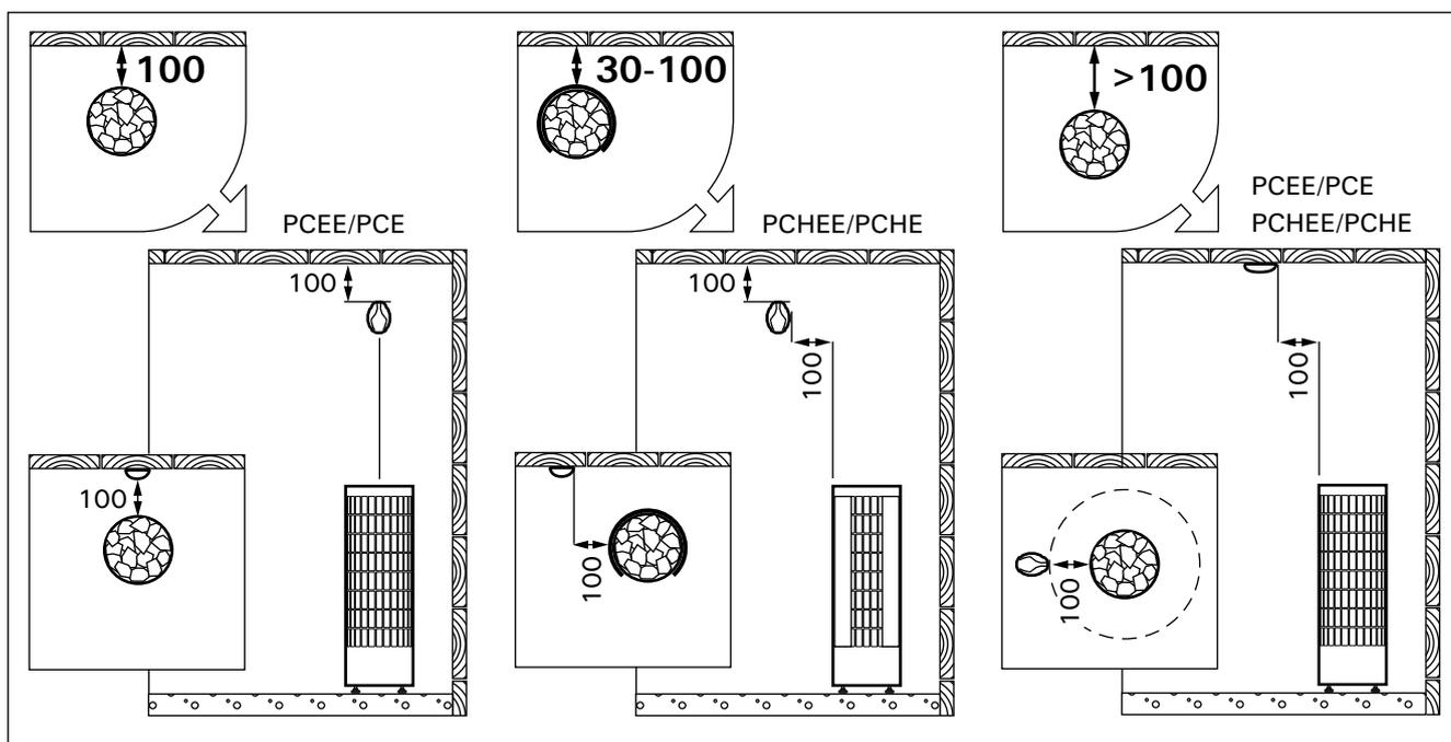
Figure 6. Installing the temperature sensor (all dimensions in millimeters)
